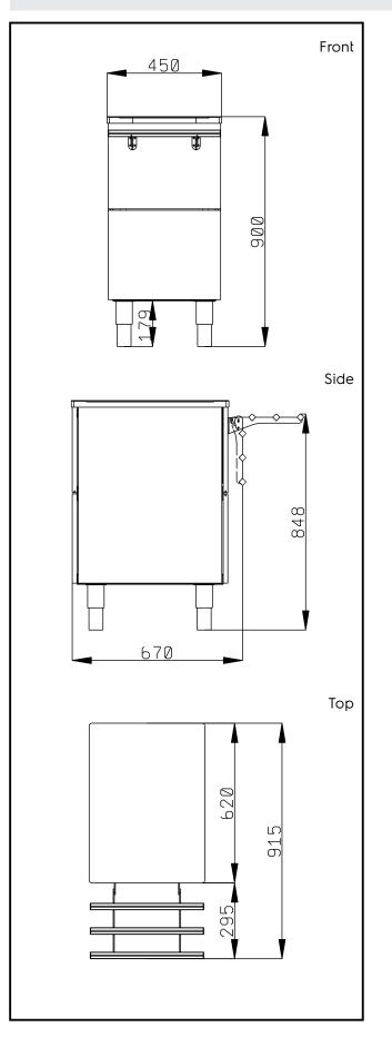
Flexy Compact Ambient Unit on cupboard (1 GN) with one stainless steel tray slider
